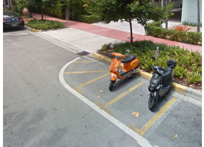
Motorcycle parking is often allowed adjacent to curb cuts and intersections. Bicycle parking should be an additional option.
