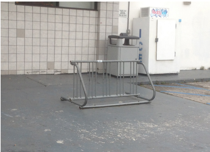
The "comb rack" is not desired because they are difficult to use and do not bicycles efficiently.
