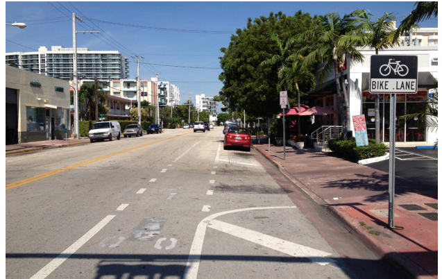
The 16th Street bicycle lane, west of Alton Rd. The use of dashed lines adjacent to the parking lot entrance marks a potential conflict point for motorists and cyclists.
